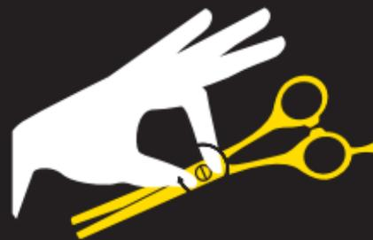
**EN - How to Check:** Hold the scissors between your thumb and index finger and tap lightly with the fist of the opposite hand.
