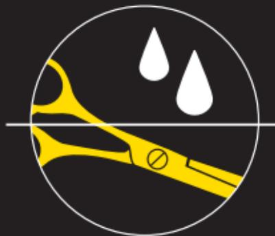
**EN -** To avoid corrosion, moisture must be wiped off the scissors thoroughly. If rust is found on the scissors, send them in immediately for repair to avoid further damage.
