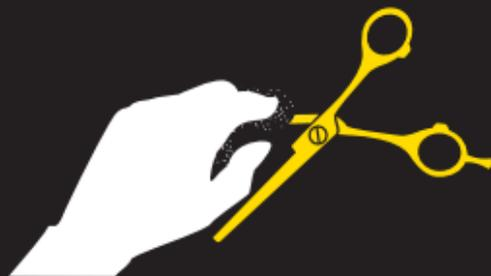
**EN** - To remove invisible unevenness, hold and wipe the scissor blades from bottom to tip with the chamois leather cloth included with your Barnum scissors. Be careful when wiping not to injure your fingers or to cut the leather.
