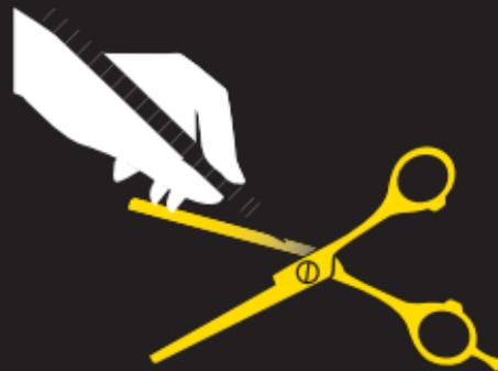
**EN** - Use the Barnum Scissors oil pen to coat the scissors' joint area and backside of the blades to ensure smooth cutting, antirust effect and long-life.
